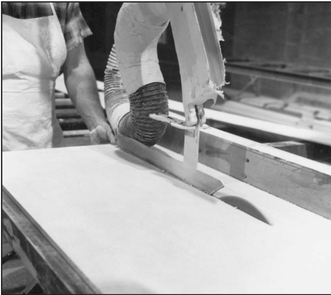
Straight line sawing (vacuum hood raised).
