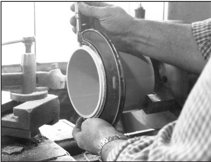
When turning fiberglass on a lathe, set the cutter slightly above center to reduce tearing action on the glass fibers.
